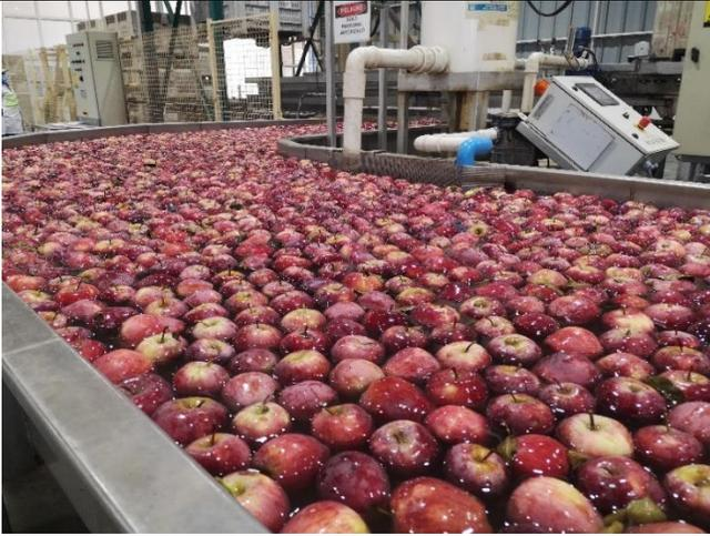
Apples harvested in bins are mechanically placed in the selection line.
